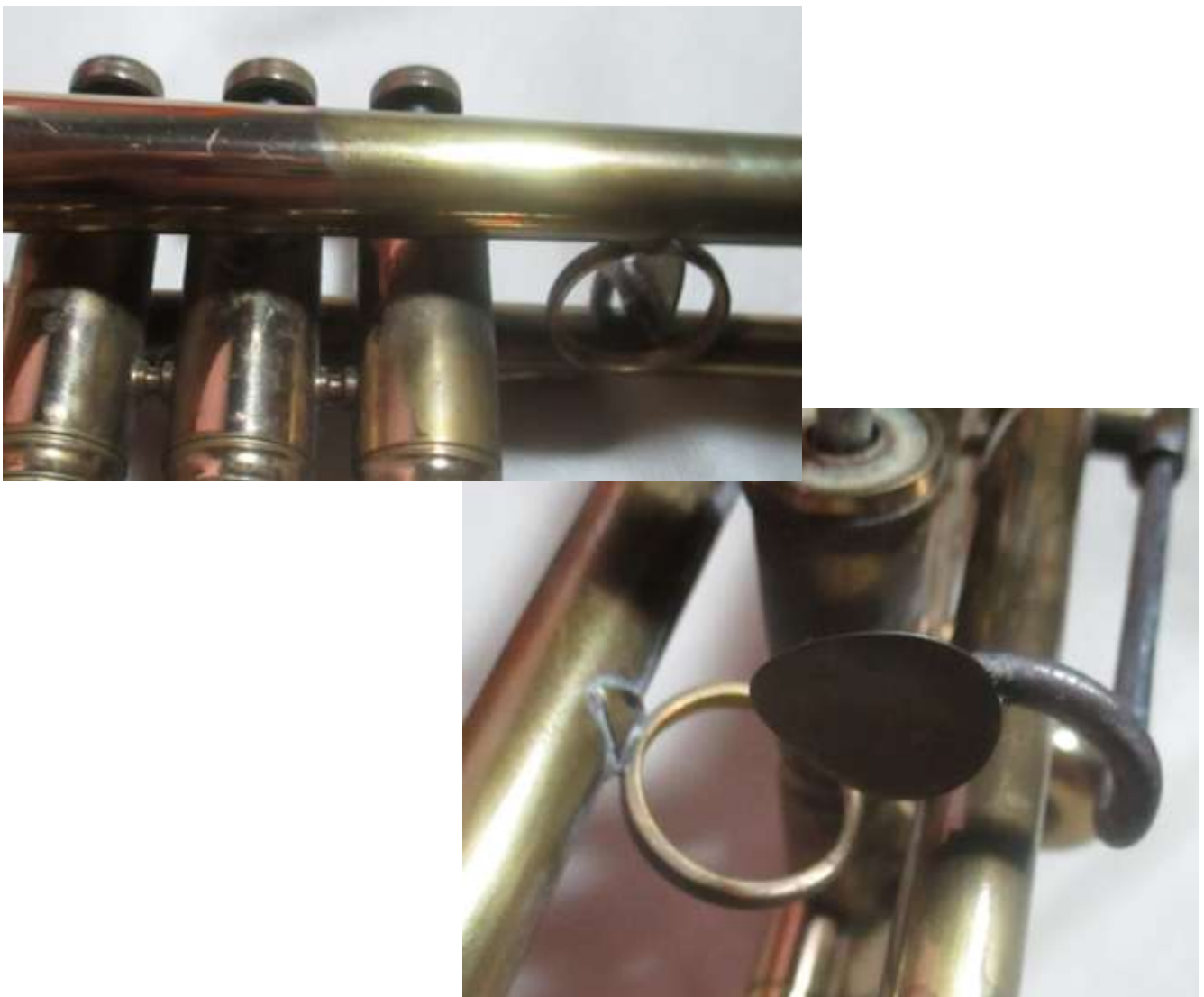
Fig. 8: Relocation of Third Valve Tuning Slide Ring.
