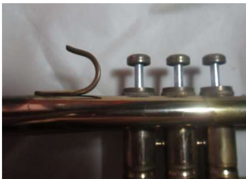
Fig. 1: Relocation of Finger Hook.
